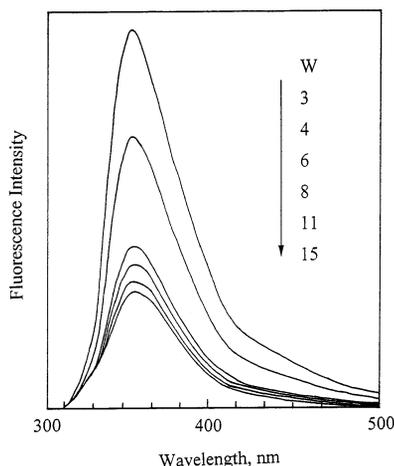
Fig. 1. Fluorescence spectra of DMABOA in AOT/cyclohexane/H<sub>2</sub>O reverse micelles [AOT] = 0.05 mol/l, [DMABOA] =  $2.5 \times 10^{-5}$  mol/l.
