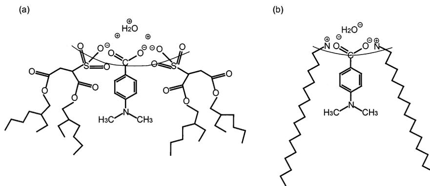
Scheme 1. The schematic picture for solubilization region of DMABOA in (a) AOT and (b) CTAB reverse micelles
