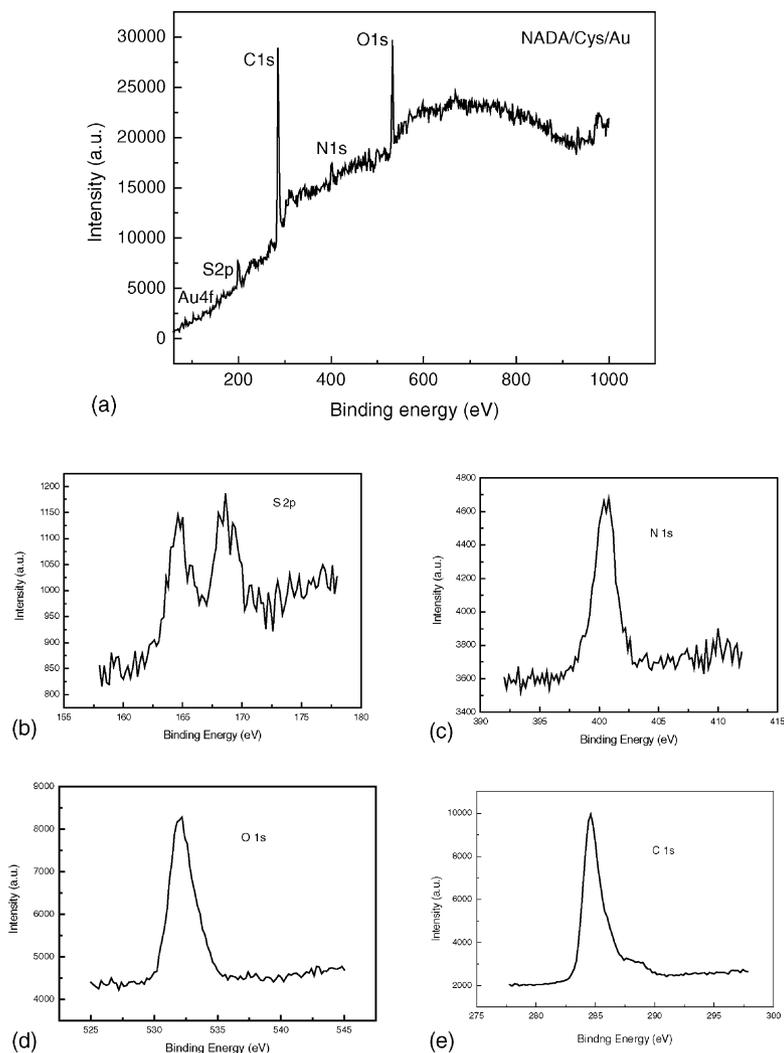
Fig. 3. XPS of NADA/Cys/Au electrode. (a) Wide view, (b) S 2p spectrum, (c) N 1s spectrum, (d) O 1s spectrum, and (e) C 1s spectrum.
