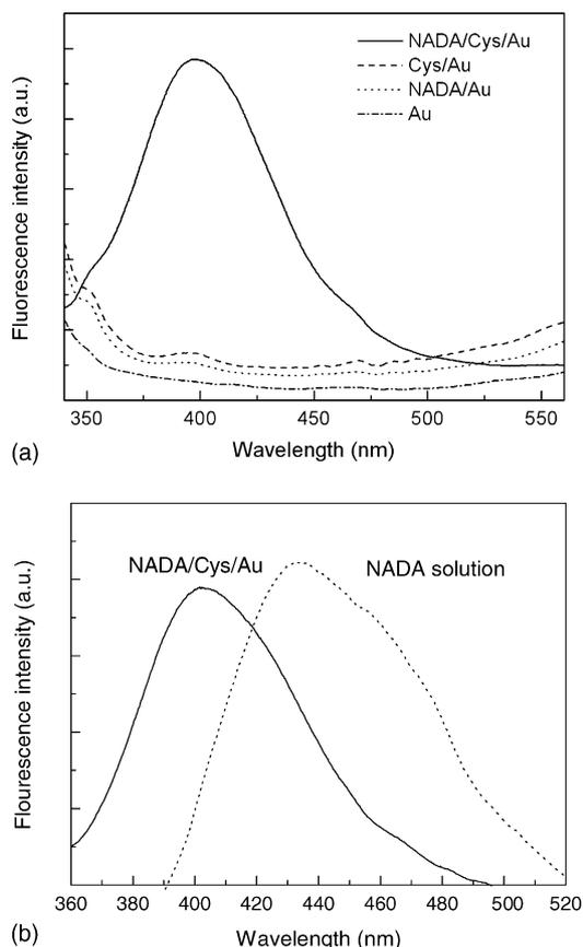
Fig. 6. (a) Surface fluorescence spectra of NADA/Cys/Au, Cys/Au, NADA/Au, and blank Au electrodes and (b) fluorescence spectra of NADA/Cys/Au electrode and NADA solution of pH 6. The “emission signals” shown in (a) for Cys/Au, NADA/Au, and Au electrodes are due to scattering light.
