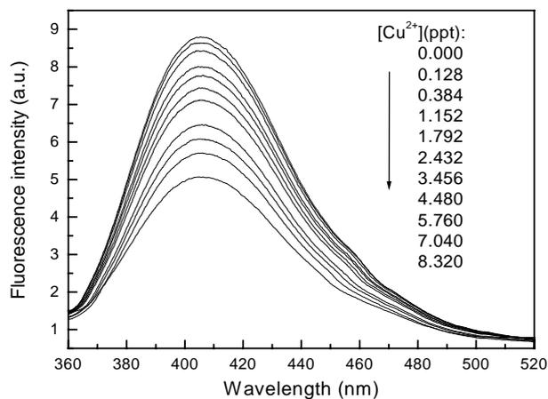
Fig. 7. Fluorescence spectra of NADA/Cys/Au electrode in aqueous solutions containing  $\text{Cu}^{2+}$  of varied concentration.
