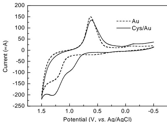
Fig. 1. Cyclic voltammograms of blank Au electrode and Cys/Au electrode in  $0.05 \text{ mol l}^{-1}$  of  $\text{Na}_2\text{B}_4\text{O}_7 \cdot 10\text{H}_2\text{O}$ – $\text{NaOH}$ – $\text{CH}_3\text{CHO}$  solution of pH 9.6. Scan rate was  $100 \text{ mV s}^{-1}$ .
