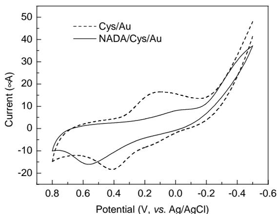
Fig. 2. Cyclic voltammograms of Cys/Au and NADA/Cys/Au electrodes in  $5 \times 10^{-4} \text{ mol l}^{-1}$   $\text{KNO}_3$  solution containing 3 ppm  $\text{Cu}^{2+}$ . Scan rate was  $100 \text{ mV s}^{-1}$ .
