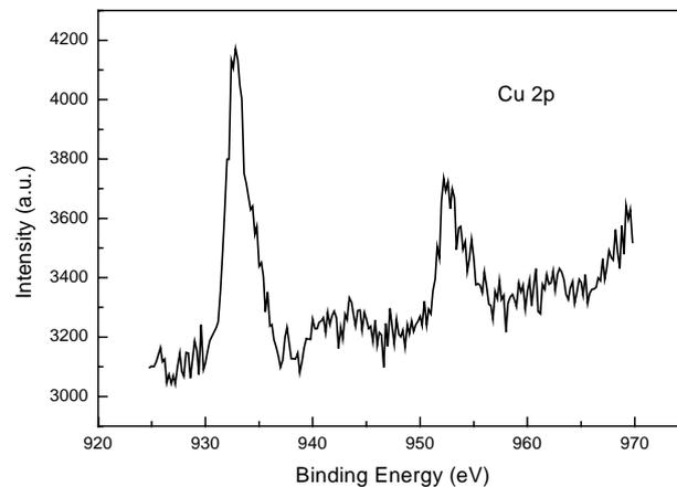
Fig. 5. Cu 2p spectrum of NADA/Cys/Au electrode after immersion in  $\text{Cu}^{2+}$  solution.
