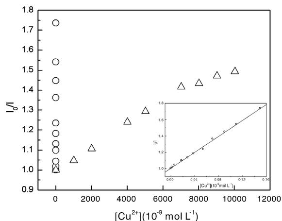
Fig. 8. Stern–Volmer plots of NADA/Cys/Au electrode and NADA solution fluorescence quenching by  $\text{Cu}^{2+}$ . (○) NADA/Cys/Au electrode in aqueous solution, (△) NADA in bulk aqueous solution. Inset shows expanded Stern–Volmer plot for the NADA/Cys/Au electrode fluorescence quenching.
