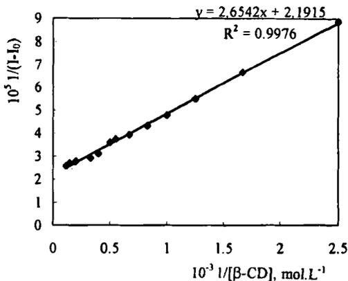
Figure 2. The double reciprocal plot of  $1/(1-I_b)$  versus  $1/[\beta\text{-CD}]$  for SDMAB/ $\beta$ -CD system.  $[\text{SDMAB}]: 2.5 \times 10^{-5} \text{mol.L}^{-1}$
