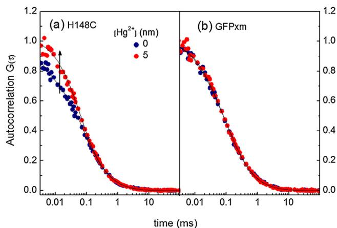
**Fig. 6.** Normalized autocorrelations  $G(\tau)$  of ca. 8 nM (a) H148C and (b) GFPxm in the absence and presence of 5 nM Hg(II) in pH 7.4 HEPES buffer at  $23 \pm 1^\circ\text{C}$ . Samples were excited by 5 mW 488-nm laser for  $10 \times 50$  s measurements. Fits are given in solid lines.
