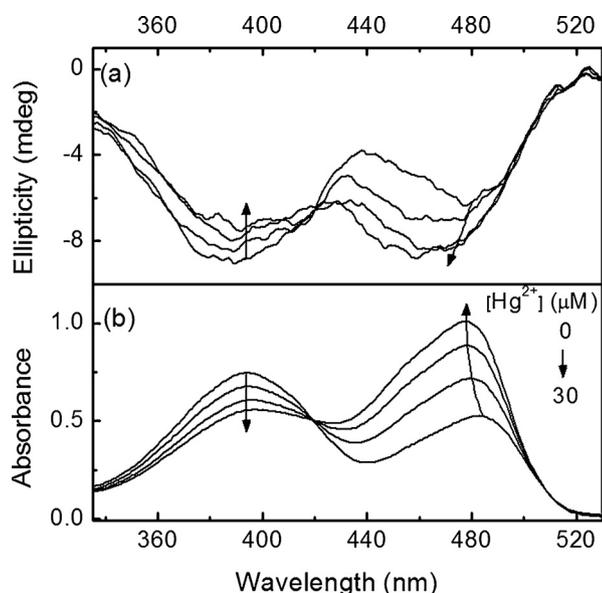
**Fig. 5.** (a) CD and (b) absorption spectra of H148C at 67  $\mu\text{M}$  with varying Hg(II) concentration (0–30  $\mu\text{M}$ ) in pH 7.4 HEPES buffer.
