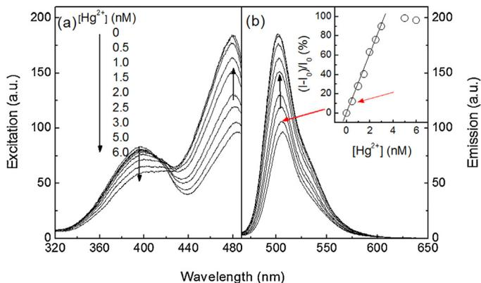
**Fig. 3.** Detection sensitivity of H148C. (a) Excitation and (b) emission spectra of H148C at 8 nM with varying Hg(II) concentration in pH 7.4 HEPES buffer. Inset in (b) shows change in fluorescence versus [Hg(II)]. Fluorescence spectrum and intensity of H148C with 0.5 nM Hg(II) are indicated by dashed arrows.
