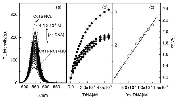
**Fig. 12** (a) PL spectra of TGA-capped CdTe NCs in 10 mM pH 7.4 Tris-HCl buffer upon addition of MB and ds-DNA of increasing concentration, (b) response plots of (●) ds-DNA, (■) C-DNA, (▼) P-DNA, (◆) I-DNA, and (▲) C-DNA and I-DNA, and (c) linear response plot of ds-DNA at low concentration. [NCs] =  $1.73 \times 10^{-7}$  M, [MB] =  $2.0 \times 10^{-6}$  M,  $\lambda_{\text{ex}} = 400$  nm.
