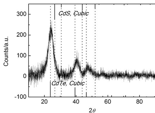
**Fig. 3** XRD pattern of TGA-capped CdTe NCs. The line spectra correspond to standard diffraction lines for cubic phase of bulk CdTe and CdS, respectively.<sup>37,42</sup>
