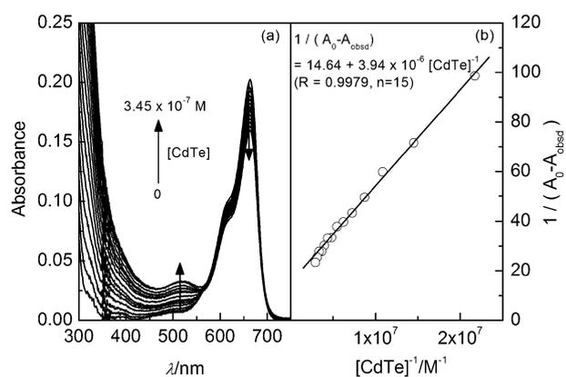
**Fig. 6** (a) Absorption spectra of MB in the presence of TGA-capped CdTe NCs and (b) double reciprocal plot of  $1/(A_0 - A_{\text{obsd}})$  versus  $1/[\text{CdTe}]$  in 10 mM Tris-HCl buffer of pH 7.4. [NCs] =  $0-3.45 \times 10^{-7}$  M, [MB] =  $2.0 \times 10^{-6}$  M.
