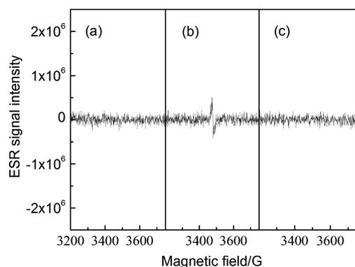
**Fig. 9** X-Band differential EPR spectra measured after UV illumination of TGA-capped CdTe NCs in the absence (a) and presence (b) of MB. Spectrum (c) is that measured after illumination of MB alone. Frequency is 9.763 GHz; UV lamp,  $\lambda < 400$  nm, 300 W.
