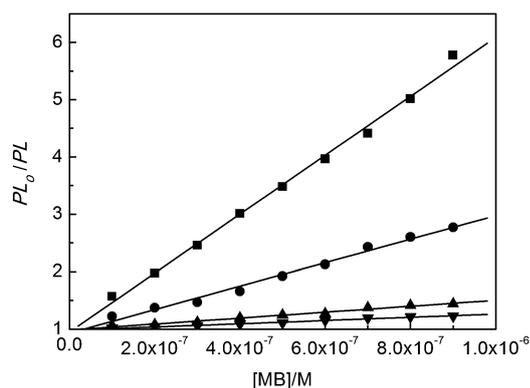
**Fig. 5** Stern–Völmer plots for quenching PL of TGA-capped CdTe NCs by MB in the presence of NaCl. [NaCl] = 0 mM (■), 10 mM (●), 50 mM (▲), 100 mM (▼). [NCs] =  $1.73 \times 10^{-7}$  M, [MB] =  $0-9.0 \times 10^{-7}$  M,  $\lambda_{\text{ex}} = 400$  nm.
