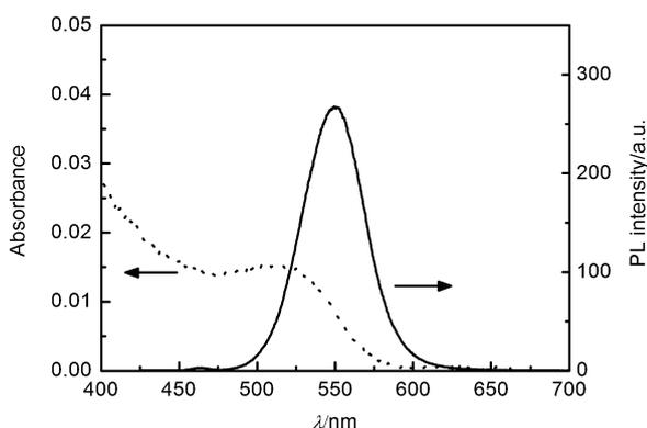
**Fig. 1** UV-vis absorption (dashed) and PL (solid) spectra of TGA-capped CdTe NCs in 10 mM Tris-HCl buffer of pH 7.4.  $[\text{NCs}] = 1.73 \times 10^{-7} \text{ M}$ ,  $\lambda_{\text{ex}} = 400 \text{ nm}$ .
