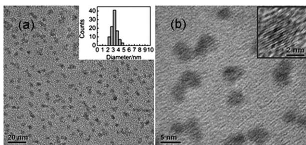
**Fig. 2** Representative HRTEM images of TGA-capped CdTe NCs. Scale bar is 20 nm (a), 5 nm (b), and 2 nm (inset in b), respectively. Inset in (a) is size distribution of TGA-capped CdTe NCs from HRTEM images.
