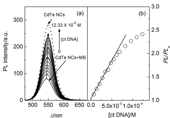
**Fig. 11** (a) PL of TGA-capped CdTe NCs in 10 mM pH 7.4 Tris-HCl buffer upon addition of MB and ct DNA and (b) ct DNA response plot obtained from (a). [NCs] =  $1.73 \times 10^{-7}$  M, [MB] =  $2.0 \times 10^{-6}$  M, [ct DNA] =  $0-12.33 \times 10^{-5}$  M,  $\lambda_{\text{ex}} = 400$  nm.
