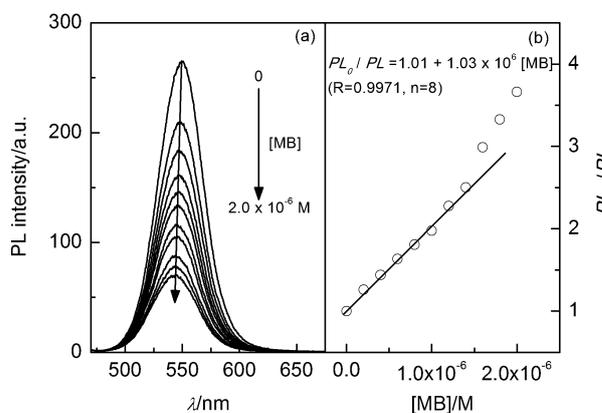
**Fig. 4** PL spectra of TGA-capped CdTe NCs in the presence of MB (a) and Stern-Völmer plot (b) in 10 mM Tris-HCl buffer of pH 7.4.  $[\text{NCs}] = 1.73 \times 10^{-7} \text{ M}$ ,  $\lambda_{\text{ex}} = 400 \text{ nm}$ .
