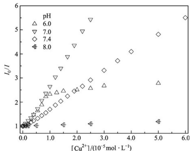
**Figure 4** Plots of  $I_0/I$  of **2** versus  $\text{Cu}^{2+}$  concentration in aqueous solution of varied pH.  $I_0$  and  $I$  are fluorescence intensities of **2** in the absence and presence of  $\text{Cu}^{2+}$ , respectively.
