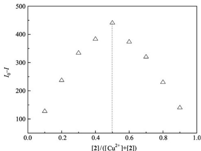
**Figure 6** The Job plot for Cu<sup>2+</sup> binding to **2** in Tris-HCl buffer (pH 7.0). Total concentration of **2** and Cu<sup>2+</sup> was  $2.0 \times 10^{-5}$  mol·L<sup>-1</sup>.
