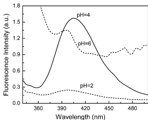
Fig. 2. Fluorescence spectra of PBA/Cys/Au obtained by dipping Cys/Au in 0.01 M PBA solutions of different pH.
