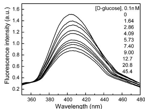
Fig. 7. Fluorescence spectra of PBA/Cys/Au in methanolic buffer solutions of pH 8.2 containing D-glucose of varied concentration.
