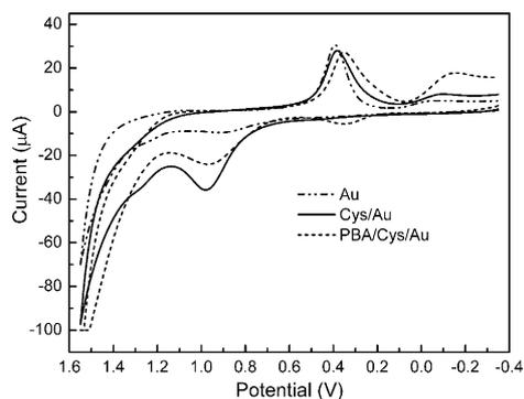
Fig. 3. Cyclic voltammograms of bare Au, Cys/Au and PBA/Cys/Au electrodes in 0.05 M  $\text{Na}_2\text{B}_4\text{O}_7\text{-NaOH-CH}_3\text{CHO}$  solution of pH 9.6. Scan rate was  $100\text{ mV s}^{-1}$ .
