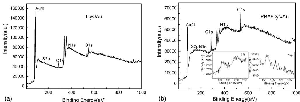
Fig. 5. XPS spectra of Cys/Au (a) and PBA/Cys/Au (b). Insets in (b) show the B1s and S2p XPS spectra.
