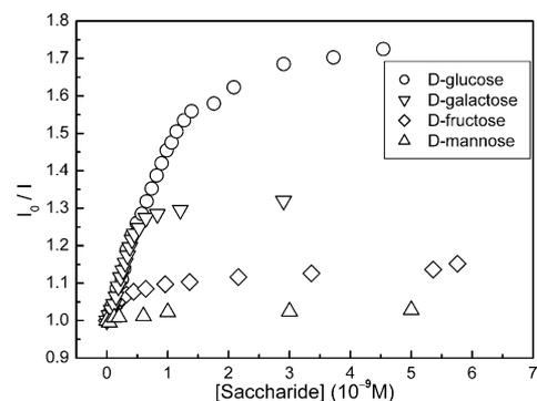
Fig. 8. Plots of the relative fluorescence intensity of PBA/Cys/Au vs. saccharide concentration in methanolic buffer solutions of pH 8.2.  $I_0$  and  $I$  represent fluorescence intensity in the absence and presence of saccharide, respectively.
