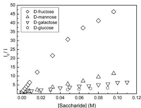
Fig. 9. Relative fluorescence intensity vs. saccharide concentration profile for PBA in methanolic buffer solution of pH 8.2. [PBA] =  $4.00 \times 10^{-4}$  M.
