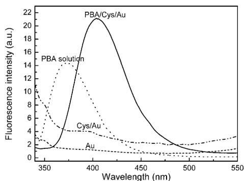
Fig. 6. Fluorescence spectra of PBA/Cys/Au, Cys/Au, bare Au wafers and PBA molecule in buffer solution of pH 8.2.
