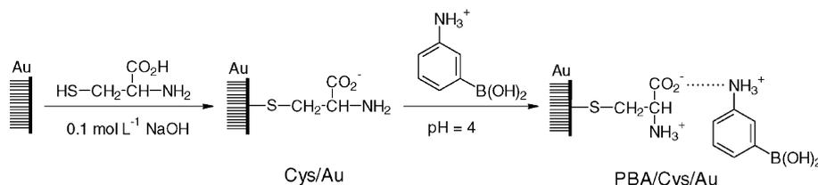
Fig. 1. Schematic diagram of self-assembling of the bilayer containing PBA.
