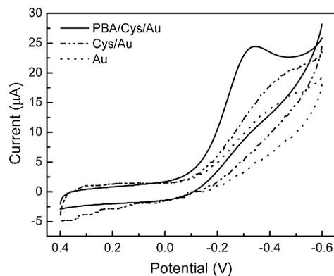
Fig. 4. Cyclic voltammograms of PBA/Cys/Au, Cys/Au and bare Au electrodes in 0.1 M  $\text{NaNO}_3$  solution of pH 2.6. Scan rate was  $100\text{ mV s}^{-1}$ .
